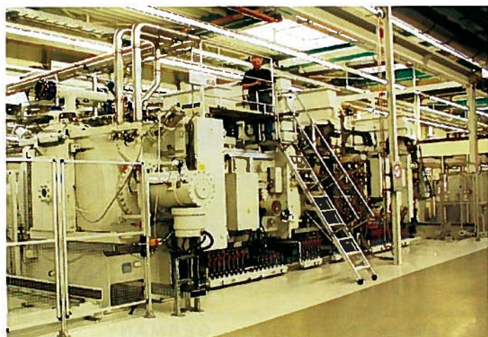
Fig. 1: Sequential vacuum hardening plant, throughput 800 kg/h
