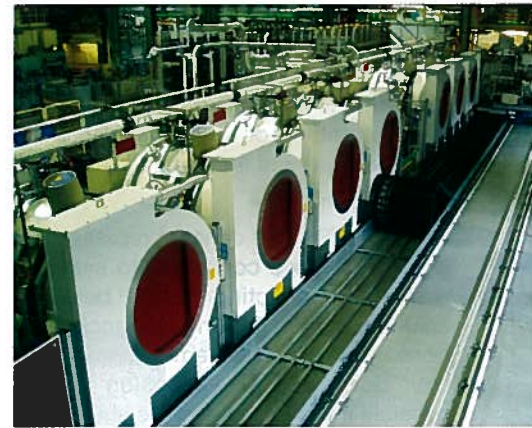
Fig. 5: Easy expanding of the modultherm-system up to 10 treatment chambers
