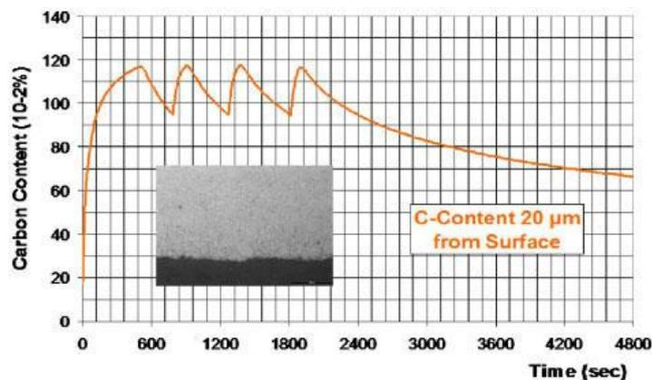
Fig 4 – Carbon Diffusion during LPC
