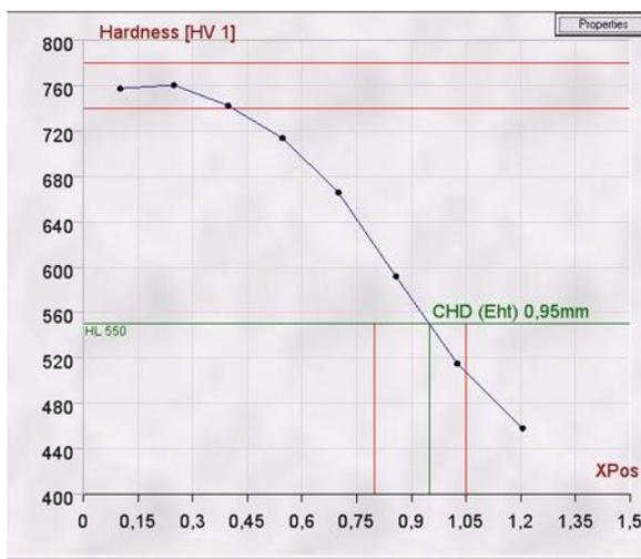
Fig 2, Hardness profile after case hardening.
