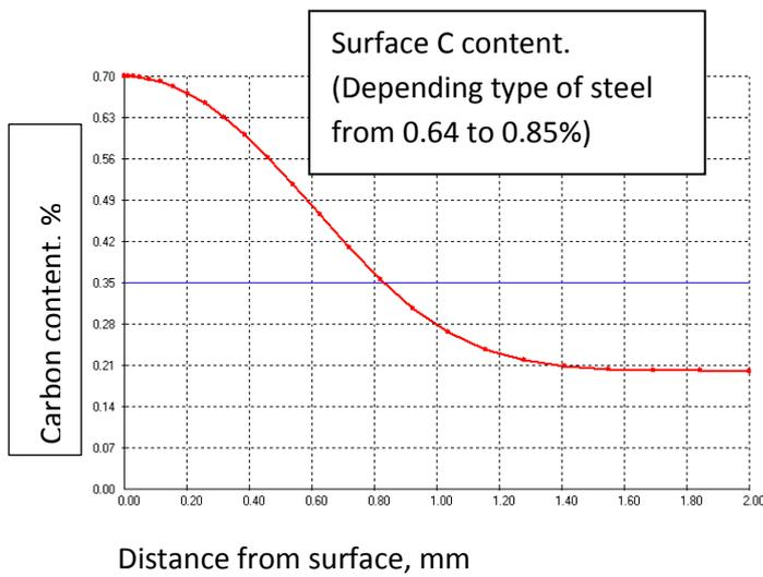
Fig 1 , Example of C profile after case hardening
