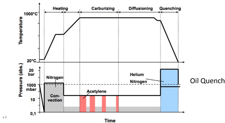
Fig 3 . Low Pressure Carburising Process Cycle
