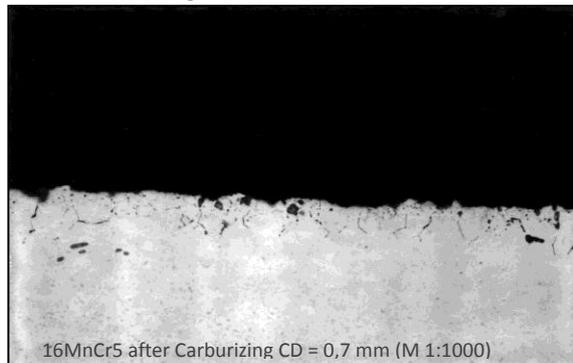
Microphotograph shown above indicates the surface of steel parts after both Low pressure carburising and Gas carburising. It clearly shows that surface after LPC process is completely free from any intergranular oxidation compared to conventional gas carburising. This further affect in reduced surface hardness, low impact and fatigue properties of parts.
