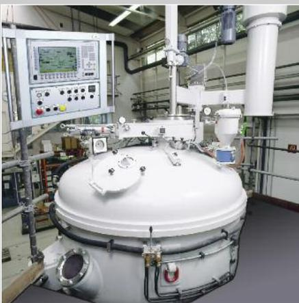
Operator platform with state-of-the-art process visualization
